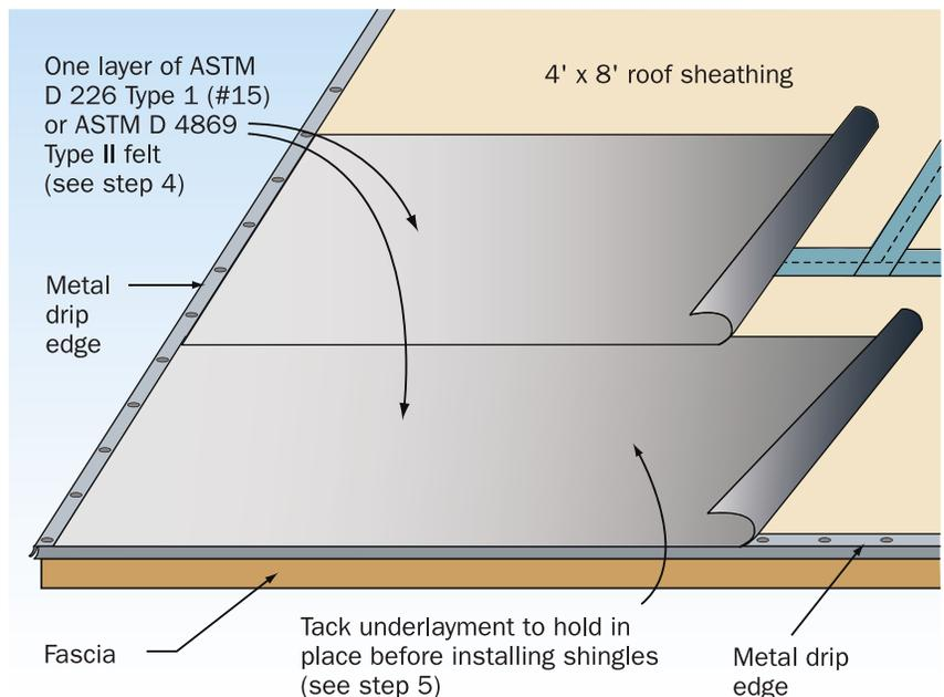
1 **Note:** If the building is within 3,000 feet of saltwater, stainless steel or hot-dip galvanized fasteners are recommended for the underlayment attachment.
