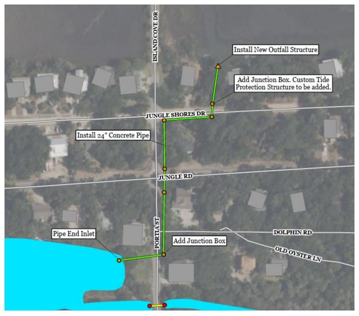
• Proposed Pipe Outfall Structure located on Portia St.
